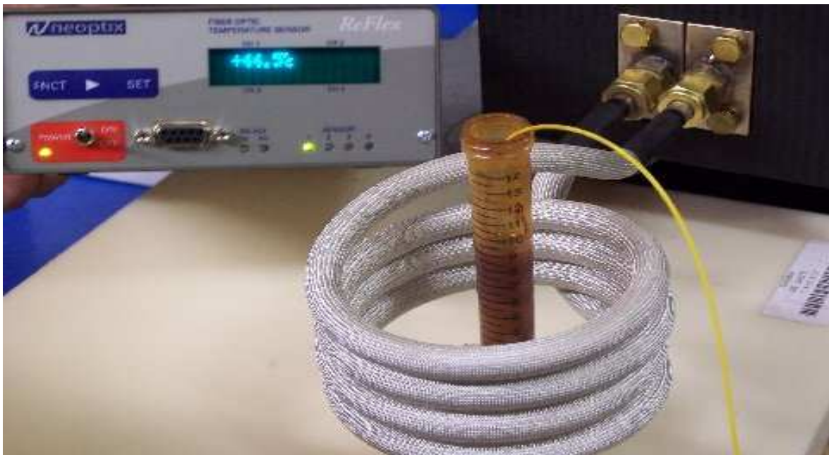
SHOWN: MEASURING FLUID TEMPERATURE WITH A FIBER OPTIC SENSING ELEMENT
